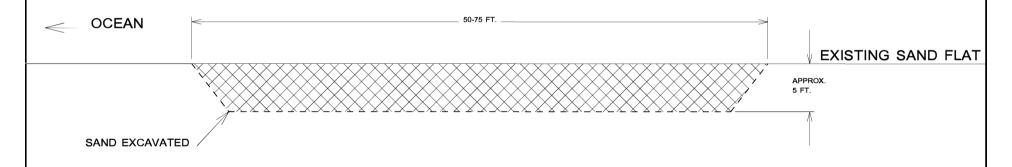
NOTE: MULTIPLE PONDS TO BE EXCAVATED TO APPROX. 5 FEET BELOW THE SAND FLAT ELEVATION. APPROX. 24,000 CUBIC YARDS OF SAND TO BE EXCAVATED.
